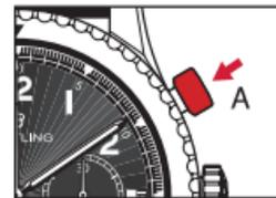
2. To interrupt the measurement, press pushpiece **A** once more. To restart the time measurement, press pushpiece **A**. This procedure makes it possible to add up several short times.
