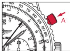
2. Stop the measurement by pressing pushpiece **A** once more. The measurement is made in hours [totalizer **1**], minutes [totalizer **2**], seconds and  $\frac{1}{4}$  of a second [hand **3**].
